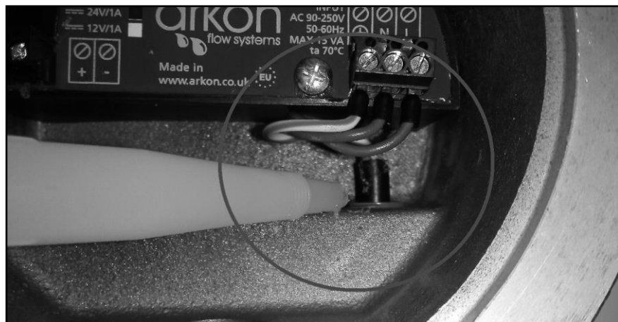
Pic. 2 Application of silicon gel on a cable of opened round cross cut cable end
